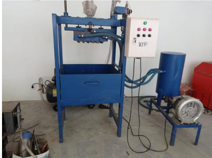
Figure 5: Egg Tray Moulding Machine
