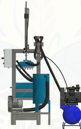
Figure 3: Egg Tray Molding Machine Design (Right View)
