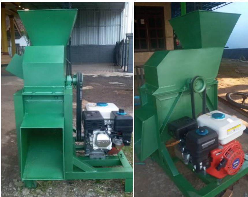
Figure 1. The designed organic waste crusher machine
