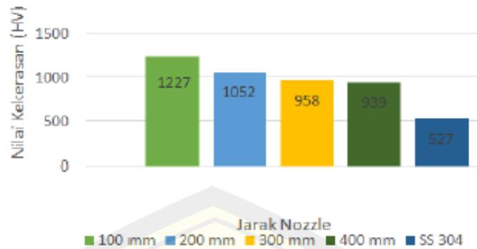
Gambar 4.10 Grafik Nilai Rata-Rata Kekerasan Substrat SS 304 pelapisan 95MXC (Sumber: Fitriyana, *et al*, 2018)
