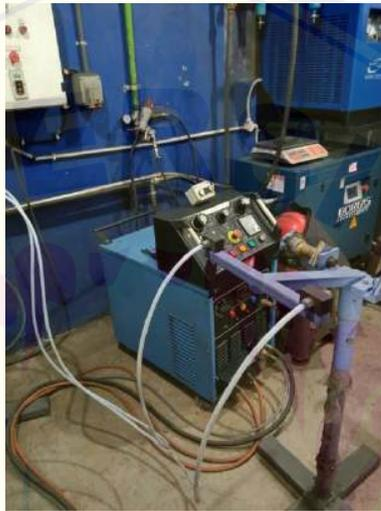
Gambar 3.1 Mesin *wire arc spray* MEC P-400 (Sumber : Dokumentasi Pribadi)
