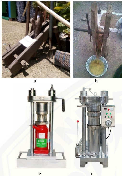
Figure 2: Ethnobotany coconut oil press (peuneurah pliek u in Acehnese regional language) (a, b) and pressurized hydraulic press (c, d) (id.aliexpress.com, 2020).
