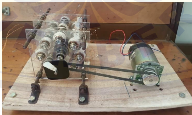
Gambar 4. 1 Generator 1 Fasa Aksial Fluks Multicakram
