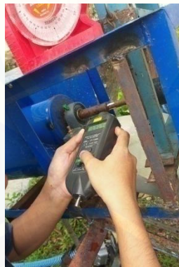
Gambar 4.3 Proses pengukuran putaran poros (Yosy, 2021)
