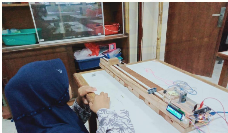
Gambar 4. 3 Proses kalibrasi sensor HC-SR04
