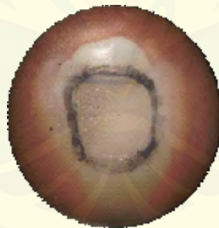
Figure 1: Observations residual adhesive material with stereo microscope.
