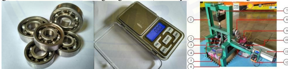
Figure 1. Rolling Resistance Test Equipment at Bearing
