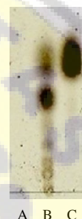
Figure 1. Result of thin layer chromatography (TLC) analysis of OPEFB-hydrolyzates. Ten percent dried-OPEFB with no buffer condition was digested by crude-enzyme 42 hours at 37°C. OPEFB-hydrolyzate with no enzyme as control (A), product (B) and glucose standards (C) was analyzed by TLC.
