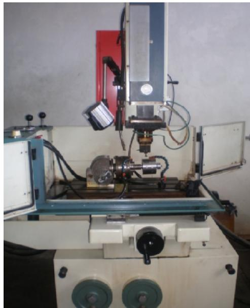
Gambar 3.3 Mesin EDM merk Jiann Sheng tipe NCF 304 N
