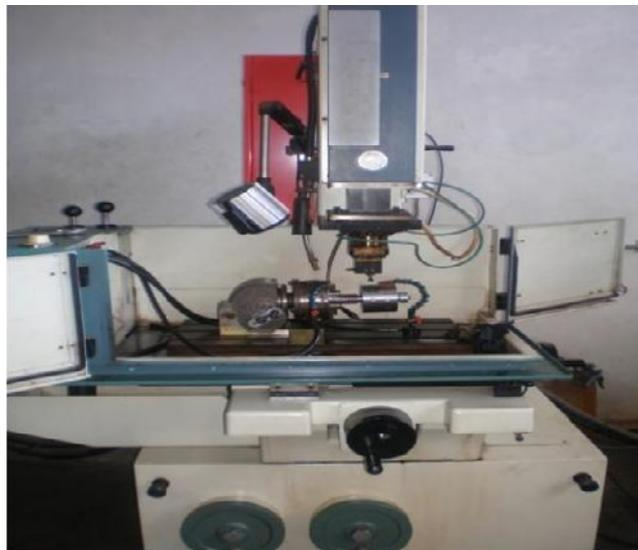
Gambar E.2 Mesin EDM *Die Sinking*
