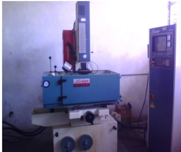
Gambar E.1 Mesin EDM *Die Sinking*
