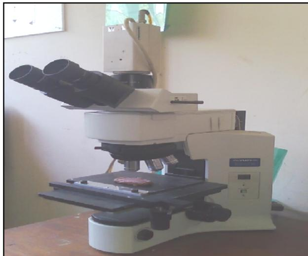
Gambar E.6 *Mikroskop Metalografi Olympus BX41M*
