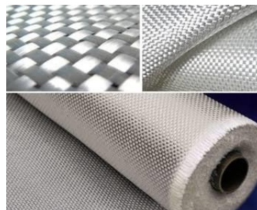
Figure 5. E-Glass Woven Roving [14]
