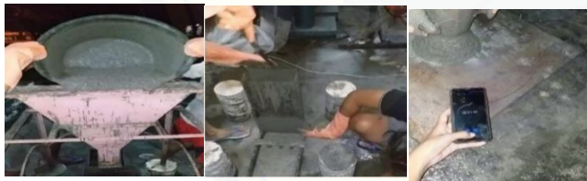
Gambar 2. Pengujian Beton Segar (a)V-Funnel, (b) L-Box, (c) Slump Flow
