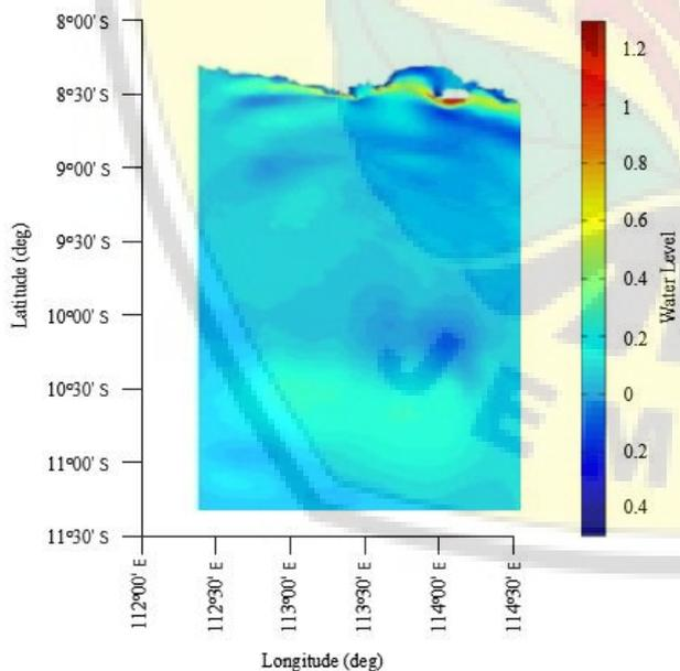
**Figure 9.** Tsunami height at minute 25 (Scenario 2)
