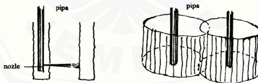
Gambar 2.6 Skema jet grouting
