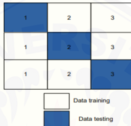
Gambar 2.3 Model 3-fold cross validation
