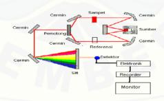
Gambar 2.13 Skema Instrumen FTIR
