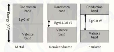
Gambar 2.2 Diagram Energi Gap setiap Material (Sumber : Molapo et al., 2012)
