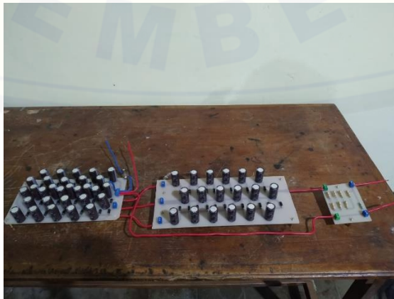
Gambar 3.9 Alat Voltage Multiplier Cockcrof-Walton 16 Tingkat Tampak Samping
