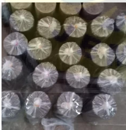
Figure 5. Curing process in ambient temperature
