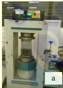
Figure 9. View of compression strength testing of concrete specimens. a) Cube 15 cm x 15 cm x 15 cm. b) Cylinder 10 cm x 15 cm. c) Cylinder 15 cm x 30 cm
