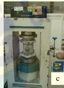
Figure 9. View of compression strength testing of concrete specimens. a) Cube 15 cm x 15 cm x 15 cm. b) Cylinder 10 cm x 15 cm. c) Cylinder 15 cm x 30 cm
