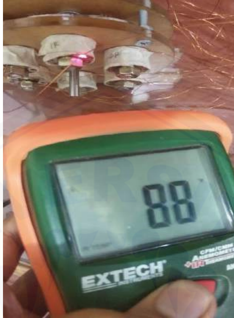
Pengukuran Suhu Setiap Kutub Enamel Motor Brushless Direct Current Axial Flux 3 Fasa Stator Ganda
