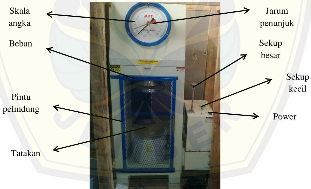
Gambar 3.2 *Material testing equipment*
