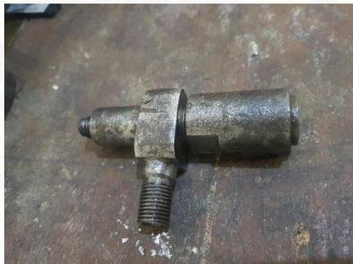
Gambar A.4 *Nozzle tipe throttle single hole*
