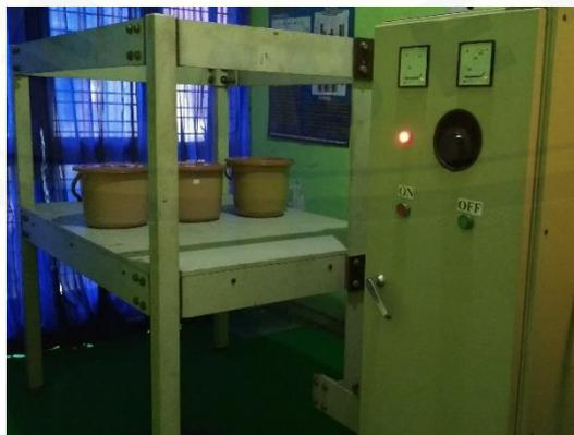
Gambar 3.2 *ELF electromagnetics Field source*
