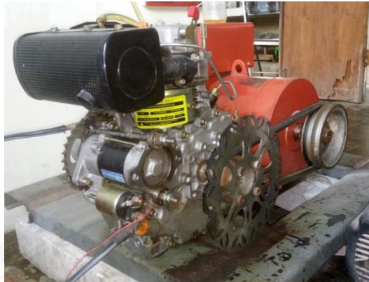
Gambar 3.1 Mesin diesel Matsumoto MDX-170 F
