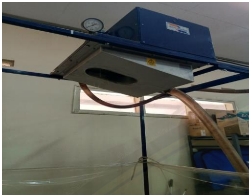
Alat rainfall simulator tipe FEL 3
