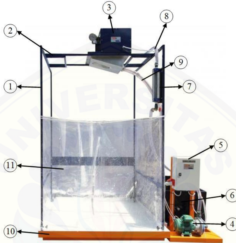
Gambar 2.3 Rainfall simulator tipe FEL3 (Sumber: Armfield, 2014)
