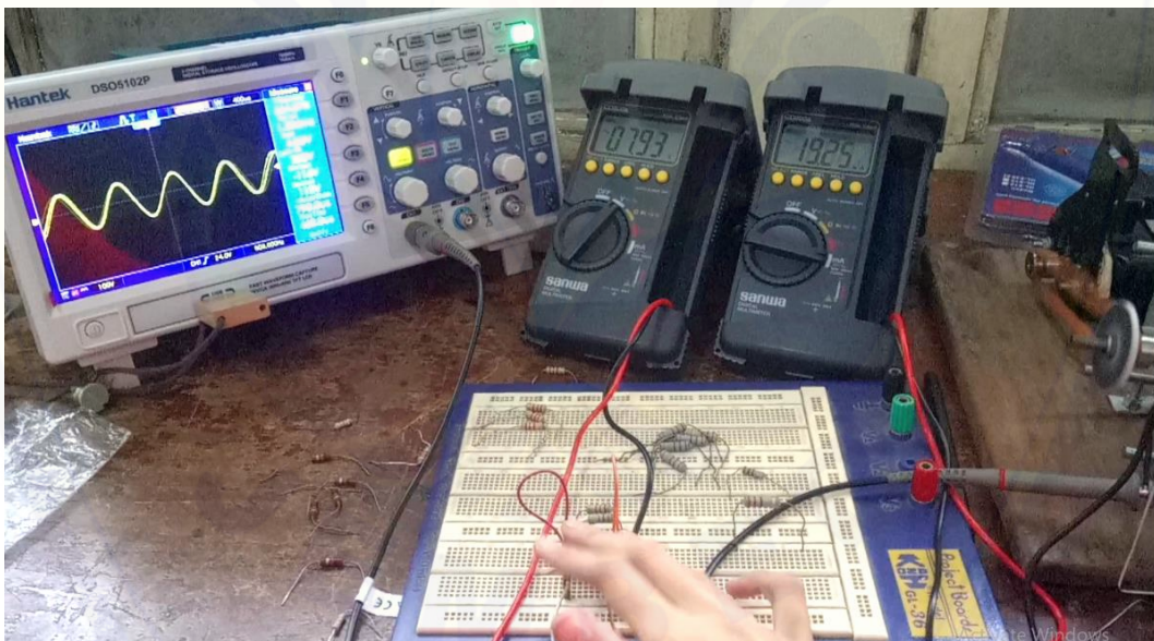
Gambar 4. Tampilan Osiloskop Pengujian Generator Axial Flux
