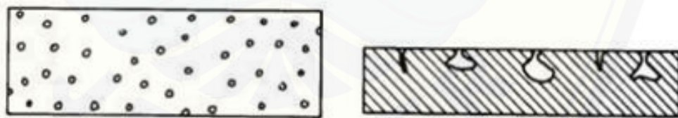
Gambar 2.3 Pitting corrosion (Sumber: TEMA, 2009)
