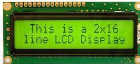
Gambar 2.5 Tampilan LCD 16 x 2
