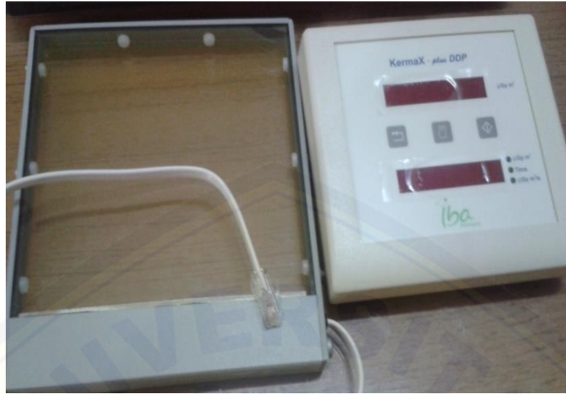
Gambar 3.2 Ionization chamber 120-131 OEM dan control/display DAP-meter tipe Kermax Plus DDP
