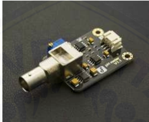
Gambar 2.7 Modul pH Value V 1.1
