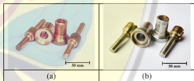
Figure-1. Types of electrodes used (a) Copper electrode; (b) HSS Electrode.
