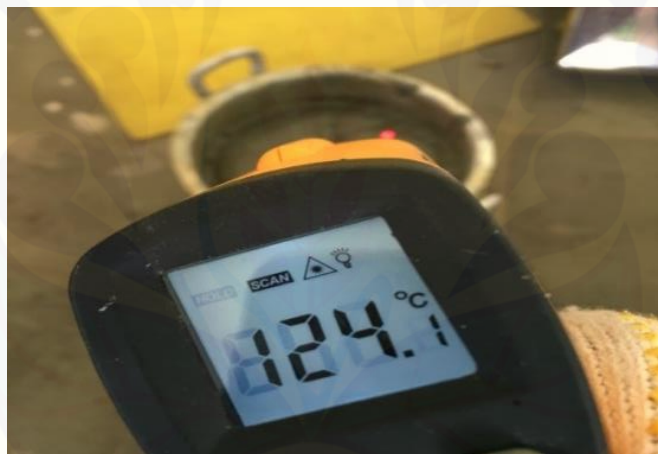
Gambar 11. Mixing tahap 2 (Pendinginan)
