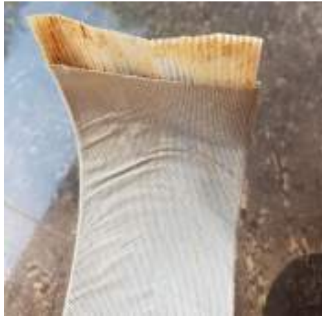
Gambar 3.2 Material Prefabricated Vertical Drain
