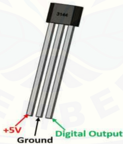
Gambar 2.4 Hall Effect Sensor (Sumber: https://components101.com/a3144-hall-effect-sensor )
