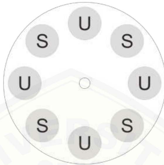
Gambar 3.3 Perancangan Rotor Brushless direct current Axial flux 8 Kutub Tampak Atas
