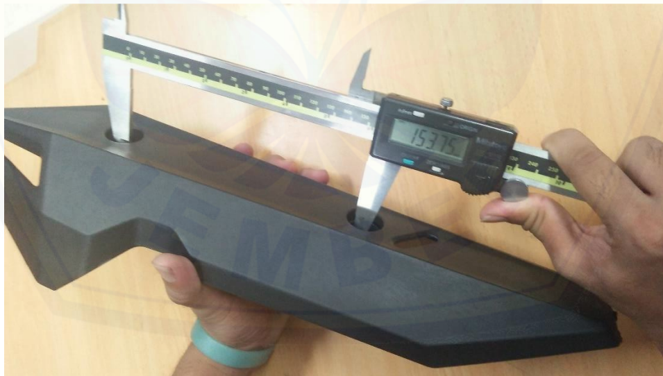
Gambar F.4 Pengukuran Shrinkage In
