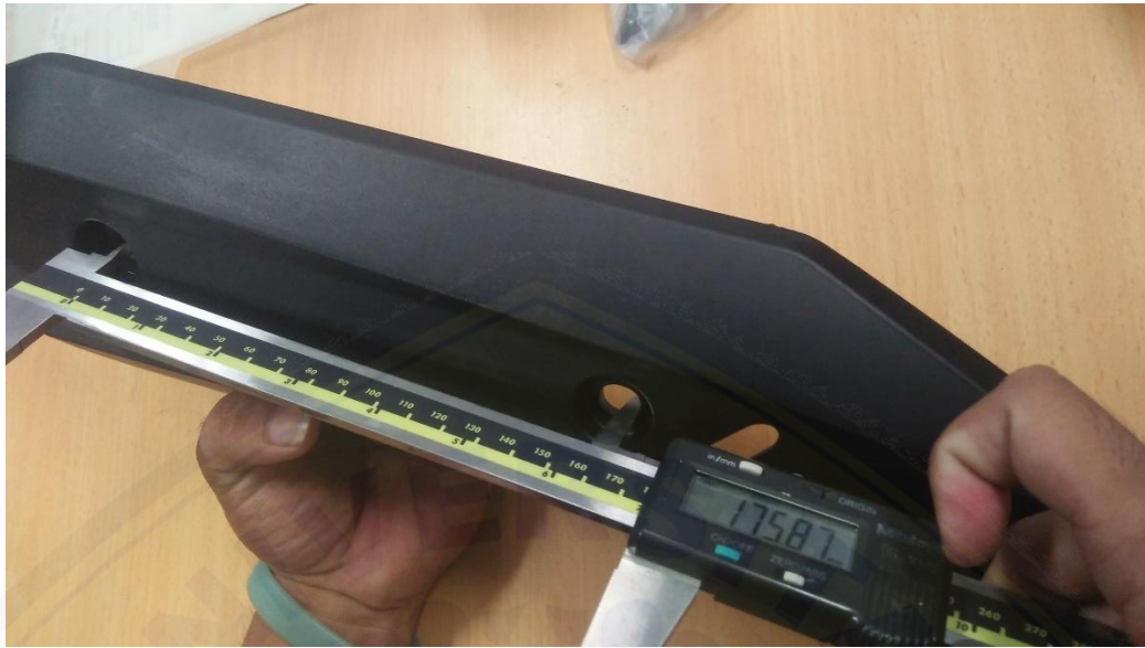
Gambar F.5 Pengukuran Shrinkage Out
