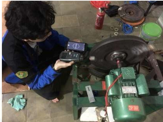
Gambar E.6 Pengujian rolling resistance
