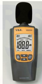
Gambar 3.1 Sound level meter (Sumber: Shanghai Yihua V&A instrument, 2005)
