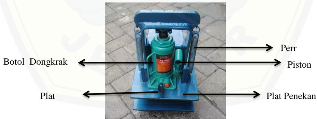
Gambar 2.6 Mesin Presss Hydrolic
