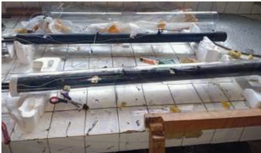
Gambar lampiran f). Pemasangan termokopel
