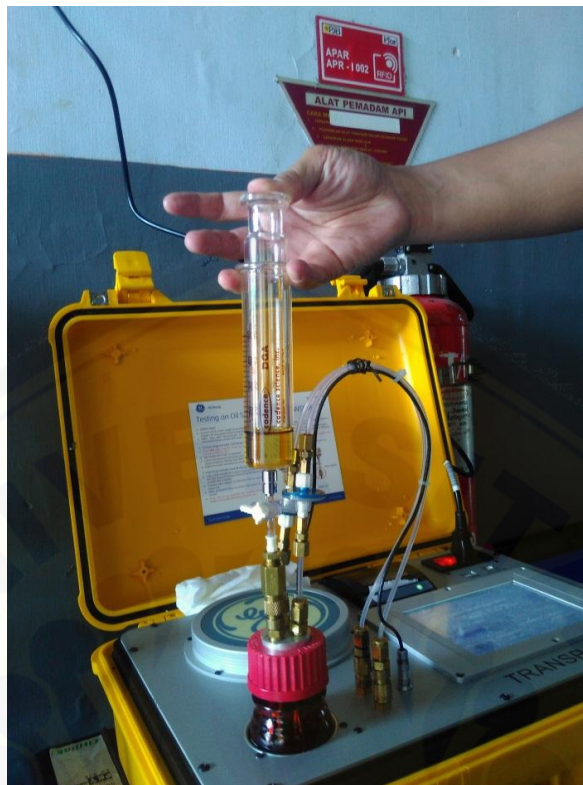
Gambar Proses Pengujian Dissolved Gas Analysis (DGA)
