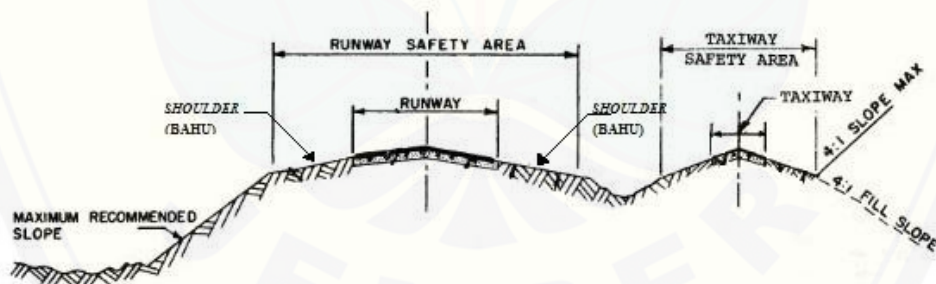
Gambar 2.4 Tampak depan elemen runway (FAA, 1989)
