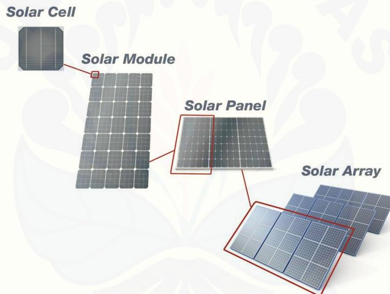
Gambar 2.1 *Solar Cell, Solar Module, Solar Panel, dan Solar Array*
