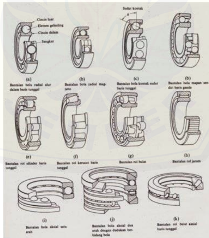
Gambar 2.8 Macam-macam bantalan gelinding (Sumber: Sularso, 1997)
