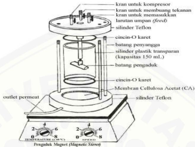
Gambar 3.3 Set Alat Ultrafiltrasi (Sumber: Irfan, 2008)
