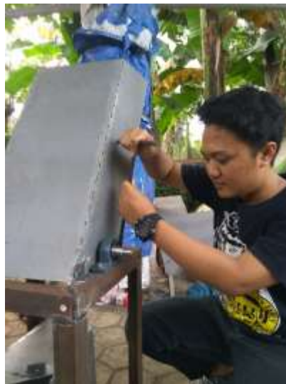
Gambar C.5 Proses pemasangan bearing
