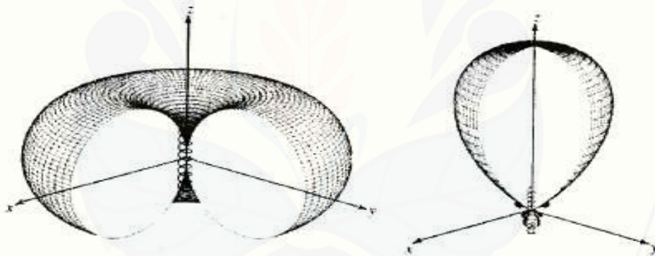
Gambar 2.6 Kiri = mode normal , kanan = mode axial
