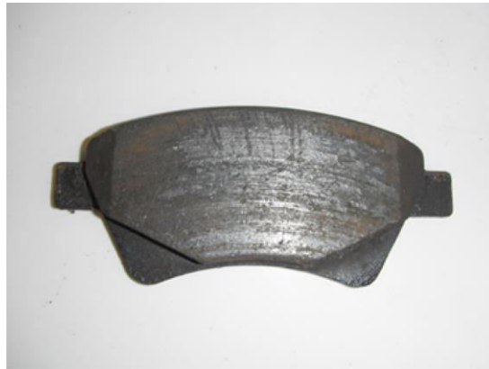
Gambar 2.13 Kampas Rem (M.C.Lagel, 2015)
