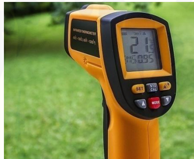
Gambar 3.3 Compact infrared thermometer with dual laser targeting
