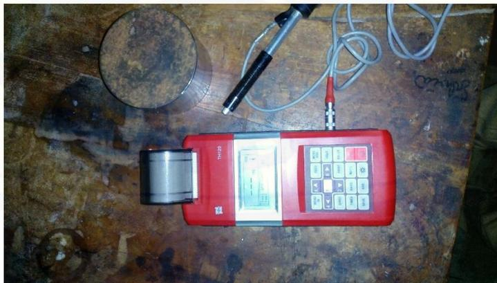
Gambar 3.3 *Hardness Tester*
